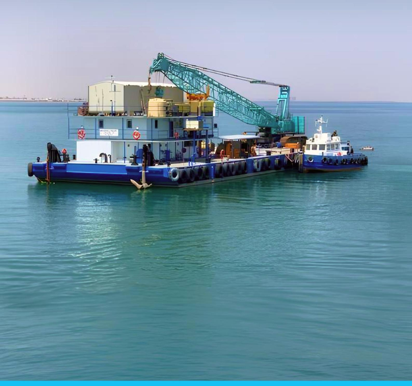
BARGE FLAT LOAD 1000 TONS
